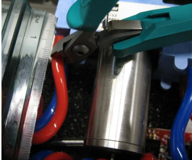
FIGURE J-9. Location of cuts to remove pump assembly from tubing
