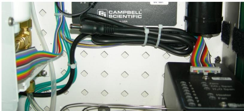
FIGURE G-2. Bundled cable of power adapter
