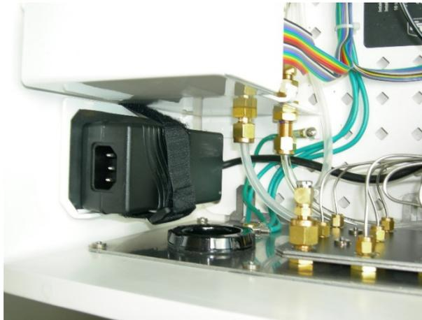
FIGURE 4-8. AC/DC power adapter kit installed in AP200
